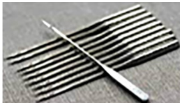
Figure 5.7: Various types of needles: (a) Sewing machine needles, (b) hand sewing needle
